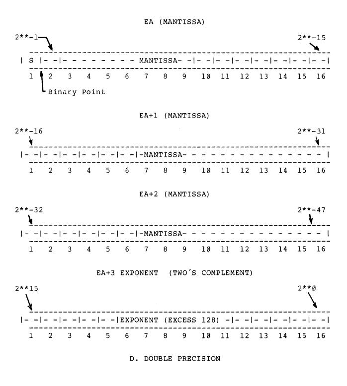
Figure 3-1. Computer Internal Word Formats for Constants and Variables (Continued)
